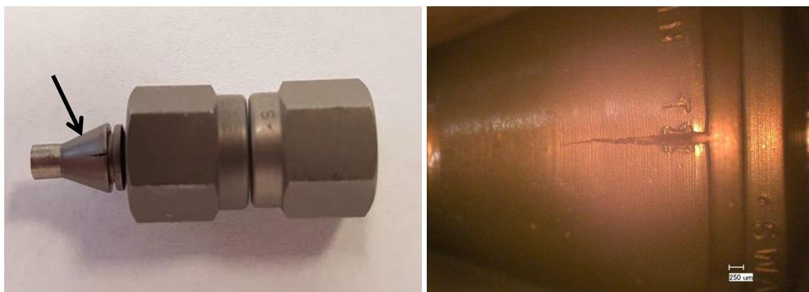
**Figure 1:** Titanium connection piece with a cutting ring crack at the position of the engraved Swagelok product number or batch.
