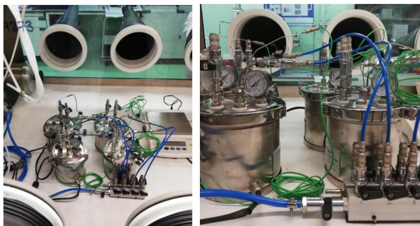
**Figure 3:** View of leaching experimental set up installed at CIEMAT in Ar glove box under 8 bar of 4.7% H<sub>2</sub>-N<sub>2</sub>.
