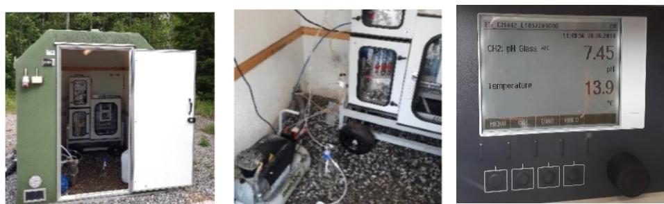
**Figure 1:** Sampling station for OL-KR6 groundwater from dept of 135 m to 137 m. The station has continuous measuring devices for most critical parameters (e.g. pH, temperature, gases) and possibility for anoxic water sampling.
