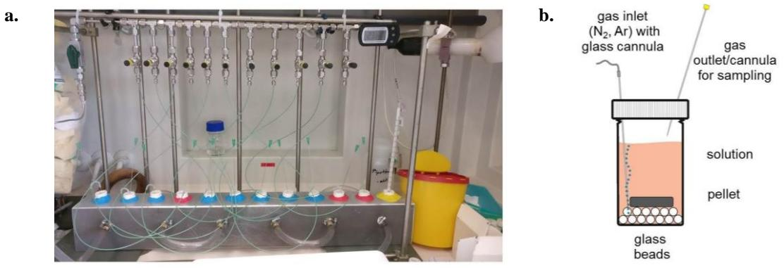
**Figure 4:** (a) Experimental setup of the dissolution experiments. (b) Schematic drawing of the experimental vessels for the accelerated dissolution experiments.
