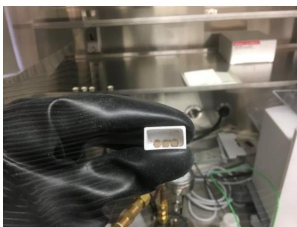
**Figure 2:** Photograph of three sintered pellets of U-Th mixed oxide handled in an anoxic glove box.
